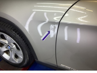
Çamurluk, sol, Çamurluk, sol > Ezik
